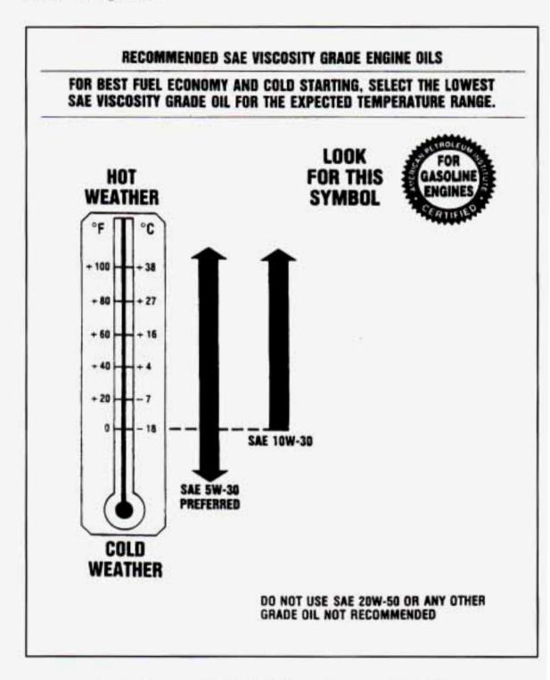
As shown in the chart, SAE 5W-30 is best for your vehicle. However, you can use SAE 10W-30 if it's going to be 0°F (-18°C) or above. These numbers on an oil container show its viscosity, or thickness. Do not use other viscosity oils, such as SAE 20W-50.
